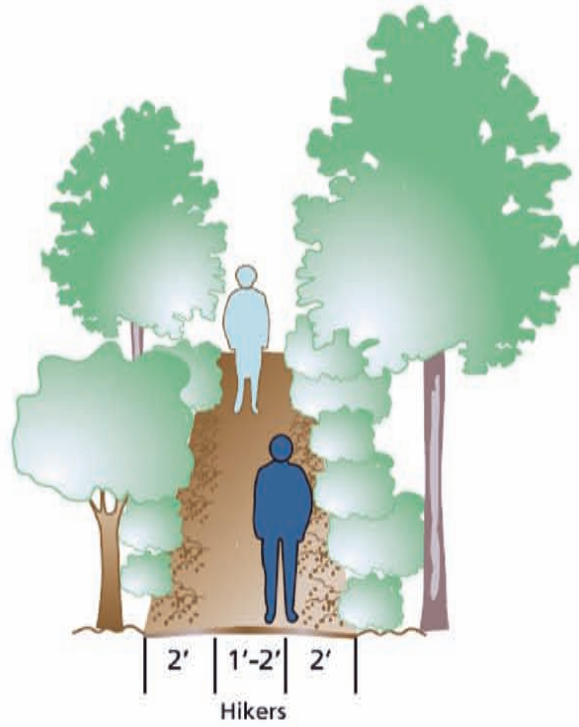
Figure X: Cross Section of a Primitive Hiking Trail
