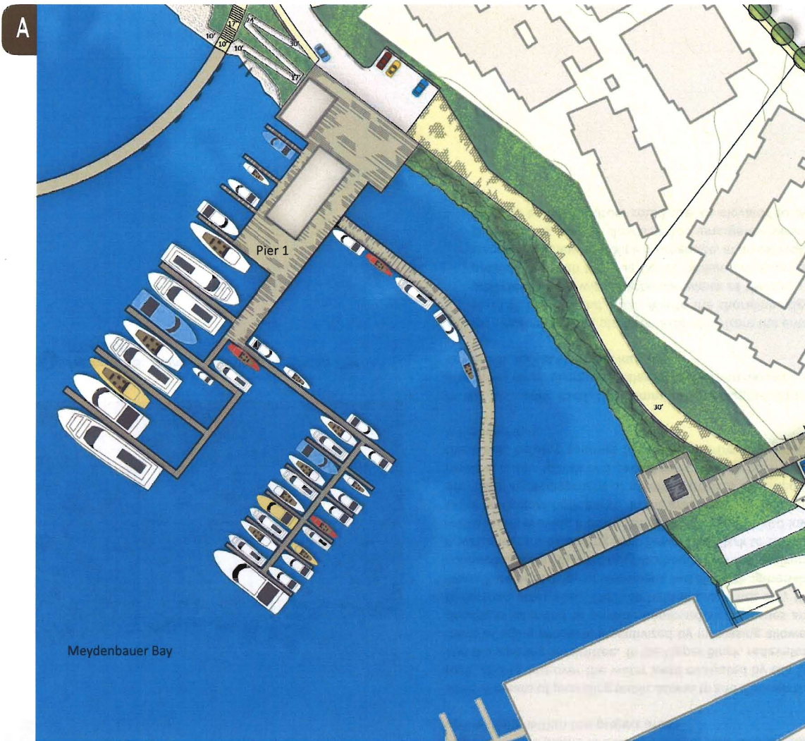
A Figure 2.5-7: Reconfigured Marina - Expanded Pier 1
