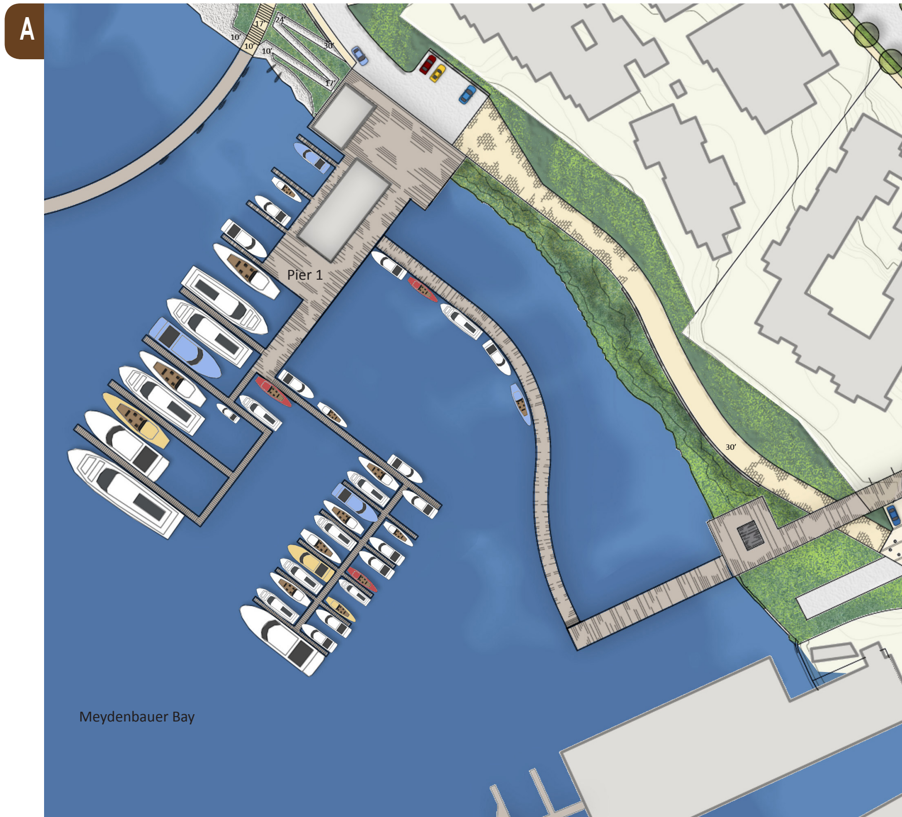
A Figure 2.5-7: Reconfigured Marina - Expanded Pier 1
