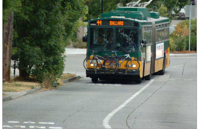
Figure 24 A bus approaches an intersection in a bus-only queue jump lane.
