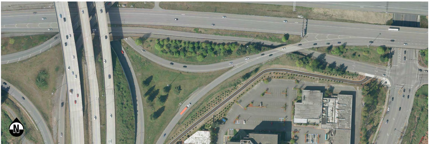
Figure 65 Running Way Improvement Project L9: The eastbound I-90 off-ramp would be widened from one lane to two by relocating the Mountains to Sound Greenway Trail. This project would help reduce signal and queuing delay caused by the signal at Factoria Blvd, helping both transit and general purpose traffic.
