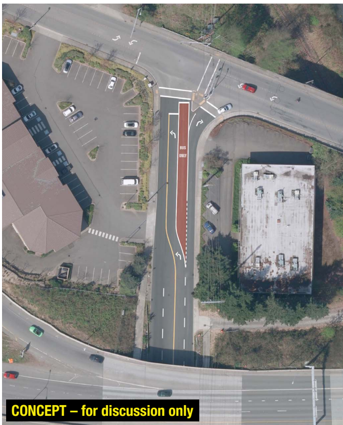
Figure 67 Spot Improvement Project Q5: Queue jump lane on NE 116th St for left turning, northeast-bound traffic at Northrup Way. Aerial images depict roadway striping before and after lane reconfiguration. This concept maintains all general purpose travel lanes and requires no new lane construction—both suitable qualities for a potential 'quick win' project.
