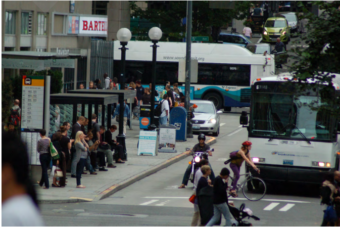
Figure 30 Curb extension on the far-side of an intersection.
