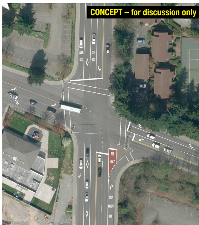
Appendix Figure 20 Spot Improvement Project Q4: Queue jump lane on 108th Ave NE for northbound buses at Northup Way. This project is no longer being considered because it cannot be accommodated by WSDOT plans currently being implemented. Also pictured is Running Way Improvement Project L17 along 108th Ave NE, a southbound HOV lane between South Kirkland Park-and-Ride and SR-520. Aerial images depict roadway striping before and after lane reconfiguration. Running Way Improvement Project L15, a BAT lane on Northup Way, is not pictured.
