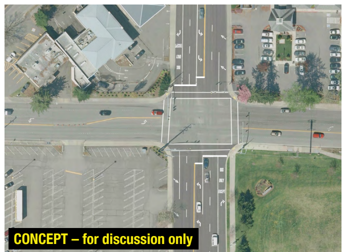
Figure 64 Running Way Improvement Projects L23 and L24: BAT lanes would be constructed on 156th Ave NE northbound from Northup Way to NE 24th St and southbound from city limits to NE 24th St, respectively. Aerial images depict roadway striping before and after lane reconfiguration. These concepts both maintain all existing general purpose travel lanes.
