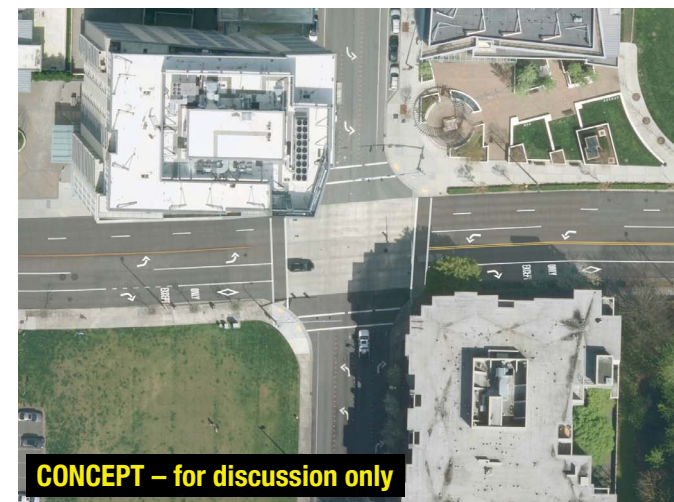
Figure 62 Running Way Improvement Project L13: PM peak-only HOV lane on NE 10th St for eastbound buses between Bellevue Way NE and NE 112th St. Aerial images depict roadway striping before and after lane reconfiguration.
