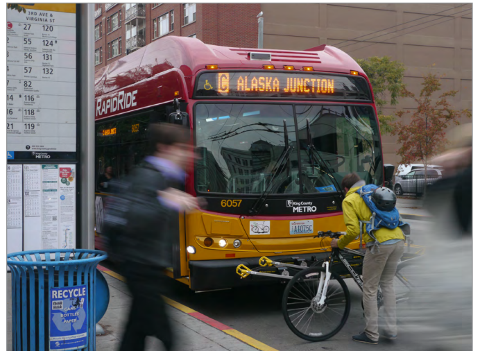
Figure 29 Unlike bull pull-outs, in-lane stops do not incur delay by requiring buses to re-enter the traffic stream.
