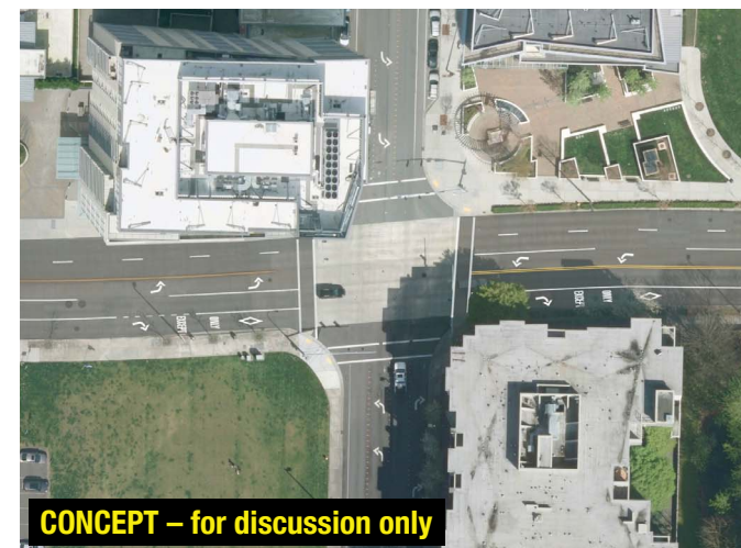
Figure 137 Running Way Improvement Project L13: PM peak-only HOV lane on NE 10th St for eastbound buses between Bellevue Way NE and NE 112th St. Aerial images depict roadway striping before and after lane reconfiguration.
