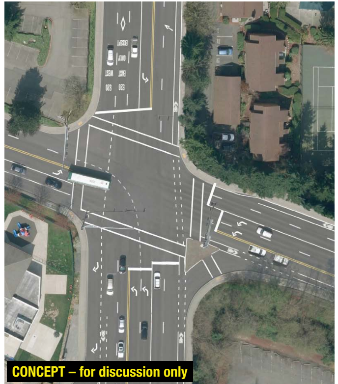
Figure 141 Running Way Improvement Project L17: Construction of a southbound HOV lane on 108th Ave NE between South Kirkland Park-and-Ride and SR-520. Aerial images depict roadway striping before and after lane reconfiguration. This concept adds one lane to the north approach relative to the WSDOT intersection reconfiguration currently being implemented. A northbound queue jump lane was also previously being considered at this intersection (see Project Q4 on page A297), but it is no longer being considered because it cannot be accommodated by WSDOT's plans.
