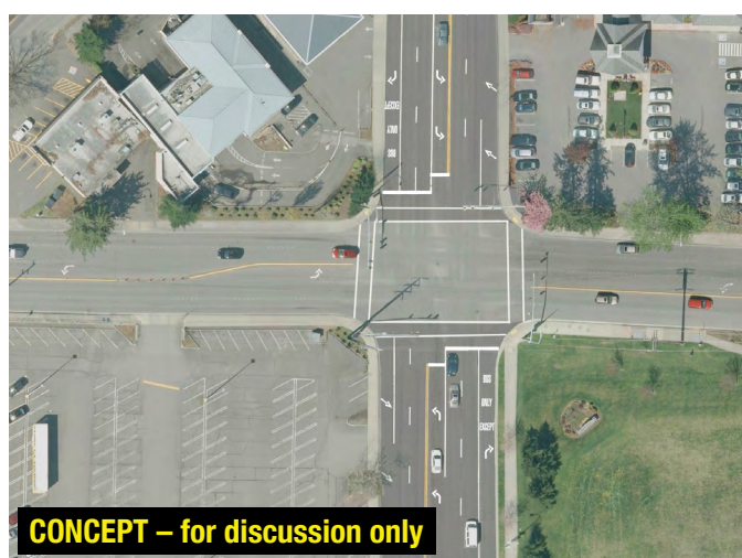
Figure 139 Running Way Improvement Projects L23 and L24: BAT lanes would be constructed on 156th Ave NE northbound from Northrup Way to NE 24th St and southbound from city limits to NE 24th St, respectively. Aerial images depict roadway striping before and after lane reconfiguration. These concepts both maintain all existing general purpose travel lanes.
