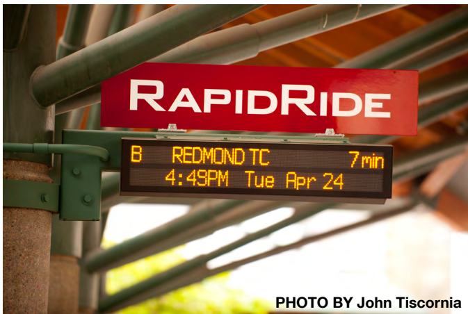
Figure 47 Real-time arrival information signboard installed by King County Metro at the Bellevue Transit Center for RapidRide B Line service.
