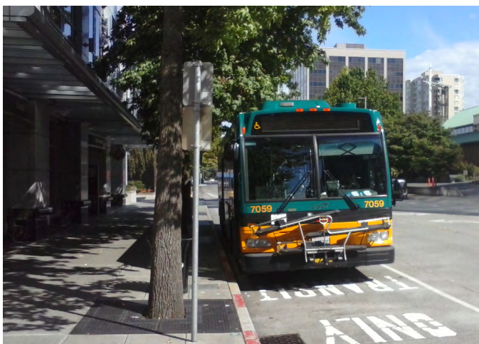
Figure 45 This stop on 108th Ave NE—Bay 1 of the Bellevue Transit Center—provides an example of a building awning providing shelter for pedestrians and waiting transit users alike.
