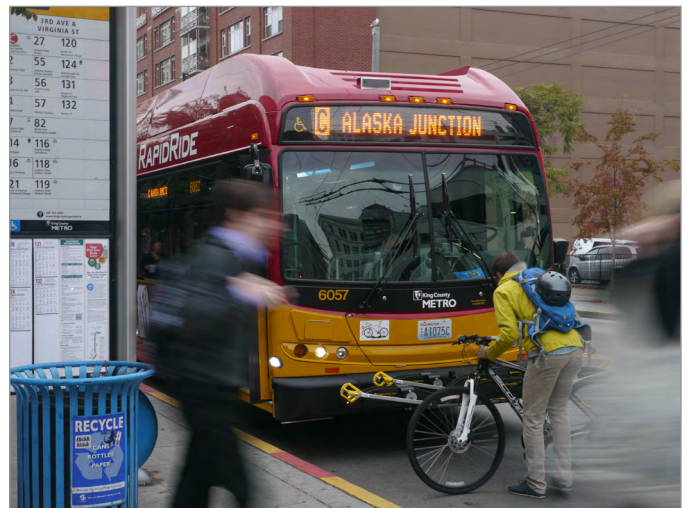
Figure 87 Unlike bus pullt-outs, in-lane stops do not incur delay by requiring buses to re-enter the traffic stream.
