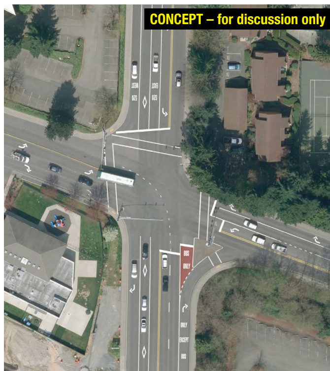
Appendix Figure 29 Spot Improvement Project Q4: Queue jump lane on 108th Ave NE for northbound buses at Northup Way. This project is no longer being considered because it cannot be accommodated by WSDOT plans currently being implemented. Also pictured is Running Way Improvement Project L17 along 108th Ave NE, a southbound HOV lane between South Kirkland Park-and-Ride and SR-520. Aerial images depict roadway striping before and after lane reconfiguration. Running Way Improvement Project L15, a BAT lane on Northup Way, is not pictured.
