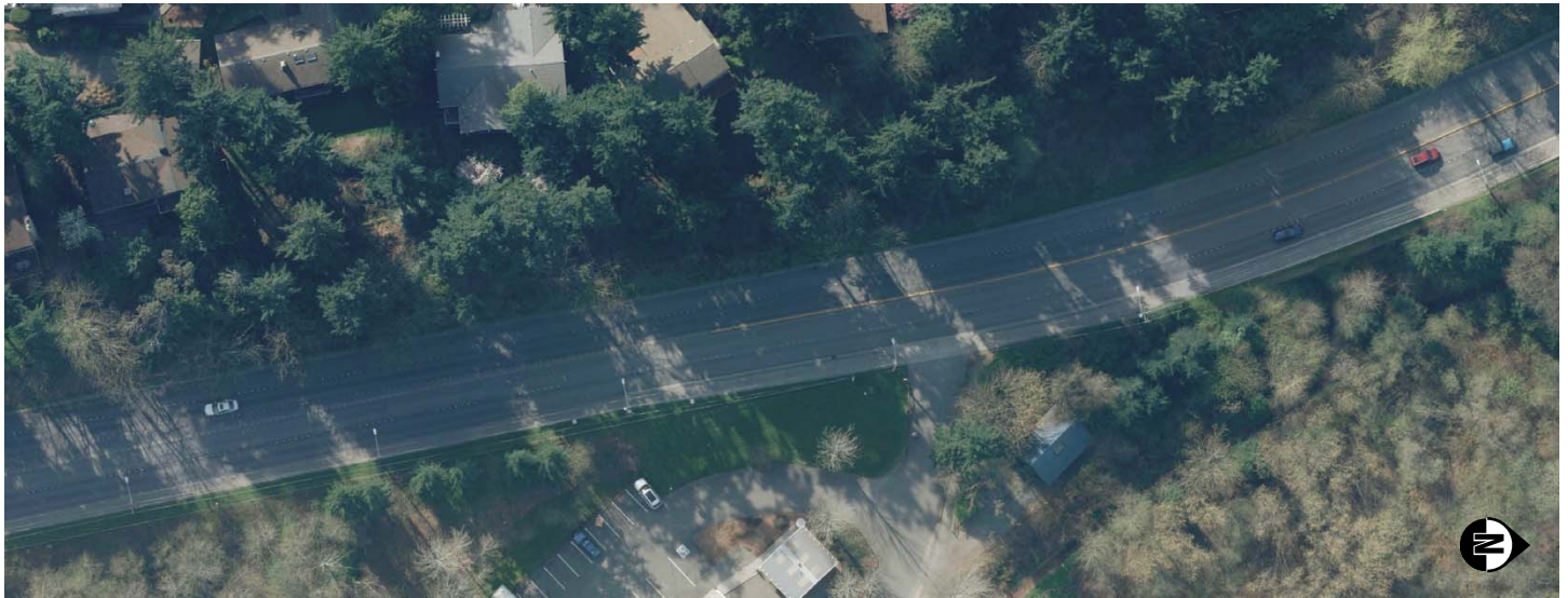
Figure 145 Running Way Improvement Projects L2: A southbound median HOV lane on Bellevue Way SE would improve the speed and reliability of transit vehicles between 112th Ave SE to South Bellevue Park-and-Ride. This would be achieved by constructing one lane on Bellevue Way SE, thereby maintaining all existing general purpose travel lanes. Aerial images depict roadway striping before and after construction.
