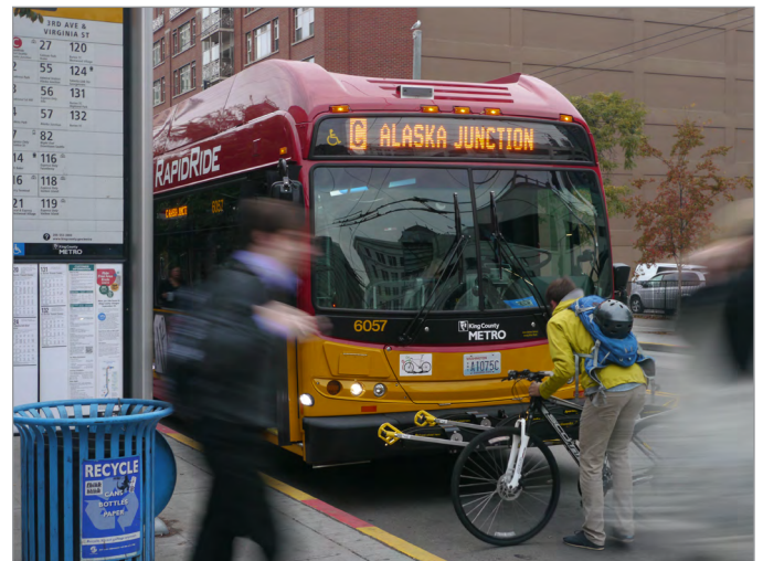
Figure 112 Unlike bus pullt-outs, in-lane stops do not incur delay by requiring buses to re-enter the traffic stream.
