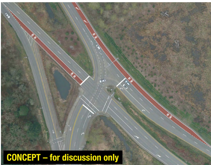
Appendix Figure 28 Running Way Improvement Project L10: A shoulder transit-only bypass lane would eliminate signal and queuing delay for northwest-bound buses on this segment of Lake Hills Connector. It is no longer being considered because adjacent wetland easements limit the available right-of-way. Also pictured is Spot Improvement Project Q11, a queue jump lane that would assist southeast-bound buses. The latter project is still being considered and would require a new lane to be constructed if implemented as shown, but all existing general purpose travel lanes would be maintained.
