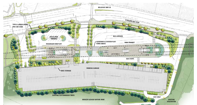
Figure 62 The 60% design of the South Bellevue Station includes designated space for bus layover and on-site bus stops for routes traveling on Bellevue Way SE.
