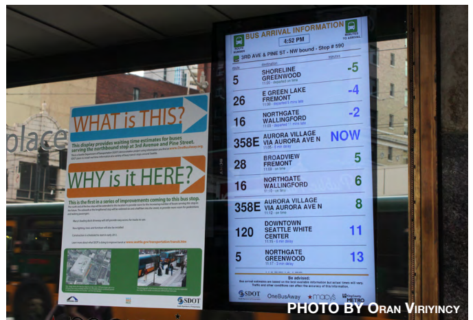
Figure 96 A digital signboard in Downtown Seattle, funded and installed by the Seattle DOT, displaying real-time arrival information from OneBusAway.
