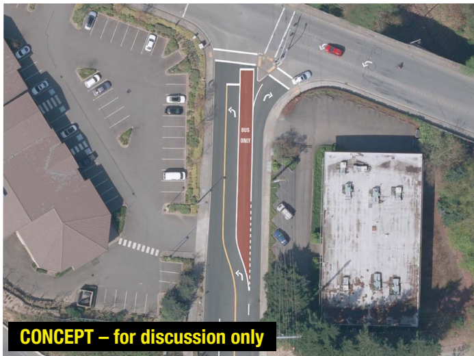
Figure 106 Spot Improvement Project Q5: Queue jump lane on NE 116th St for left turning, northeast-bound traffic at Northrup Way. Aerial images depict roadway striping before and after lane reconfiguration. This concept maintains all general purpose travel lanes and requires no new lane construction—both suitable qualities for a potential 'quick win' project.
