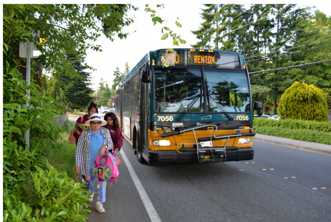
Figure 104 Users of Route 114 and 240 must walk along the shoulder to reach this bus stop (zone 65620)—southbound on 119th Ave SE just north of SE 56th St in Newport Hills, which serves about 50 ons/offers daily—because no sidewalk is provided to connect pedestrians from the intersection crosswalk to the bus.
