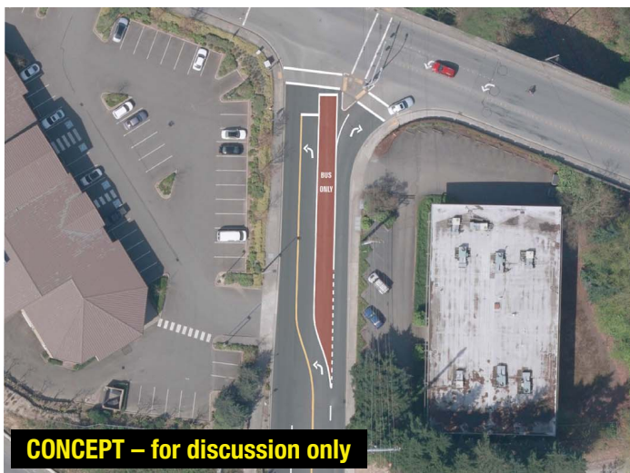
Figure 124 Spot Improvement Project Q5: Queue jump lane on NE 116th St for left turning, northeast-bound traffic at Northrup Way. Aerial images depict roadway striping before and after lane reconfiguration. This concept maintains all general purpose travel lanes and requires no new lane construction—both suitable qualities for a potential 'quick win' project.
