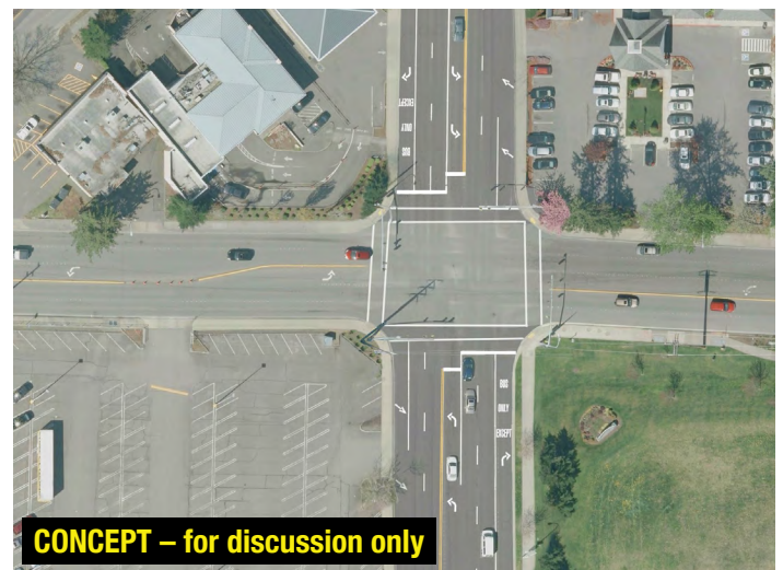
Figure 125 Running Way Improvement Projects L23 and L24: BAT lanes would be constructed on 156th Ave NE northbound from Northrup Way to NE 24th St and southbound from city limits to NE 24th St, respectively. Aerial images depict roadway striping before and after lane reconfiguration. These concepts both maintain all existing general purpose travel lanes.
