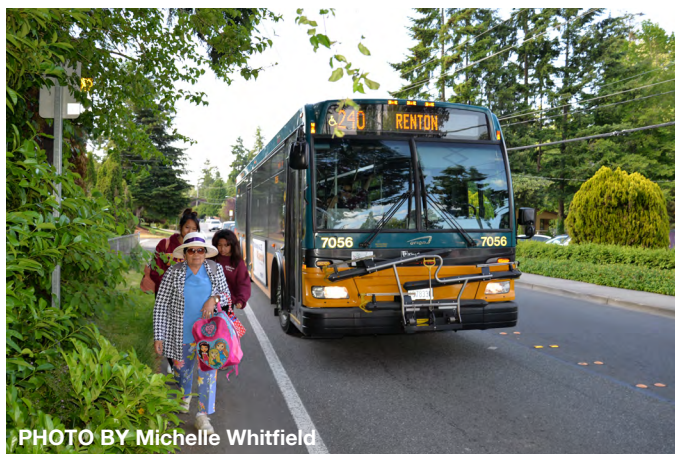
Figure 104 Users of Route 114 and 240 must walk along the shoulder to reach this bus stop (zone 65620)—southbound on 119th Ave SE just north of SE 56th St in Newport Hills, which serves about 50 ons/off daily—because no sidewalk is provided to connect pedestrians from the intersection crosswalk to the bus.
