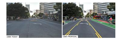
The proposed demonstration bike lane on 108th i(one of four corridors being looked at, and twhat Cascade sees as the best option) includes segments of buffered, protected and striped bike lanes. The visual above shows how 108th at 6th street (by the transit center) could be reconfigured to work for bikes, transit and cars.
