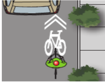
1) Shared Lane Marking
