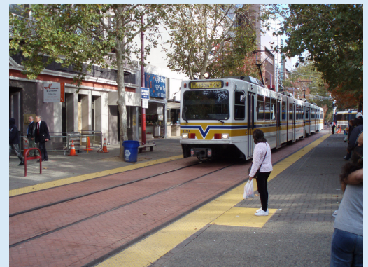
Tactile warnings and distinctive paving patterns and colors indicate to pedestrians that the zone is shared with a transit line, seen here in Sacramento, California, at St. Rose of Lima Park Station (Flickr source: Paul Kimo)..
