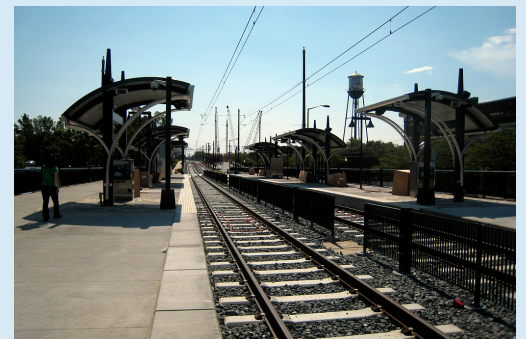
Fences can deter people from running across the tracks, shown here in Charlotte, North Carolina (Flickr source: Doug Letterman).
