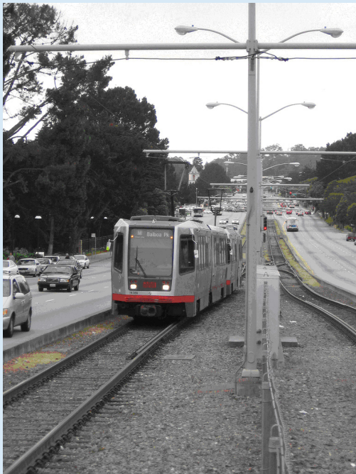
San Francisco Municipal Railway Breda light rail vehicle on the 19th Avenue exclusive right-of-way (Flickr source: Skew-T).
