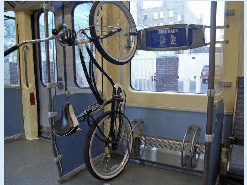
Bike racks aboard the Hiawatha light rail line in Minneapolis (Flickr source: Payton Chung).
