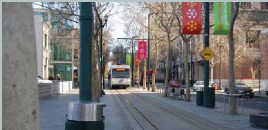
At-grade train in San Jose. Paving textures, rows of trees, street furniture and signs all help to define the train right-of-way, while creating a comfortable pedestrian environment.
