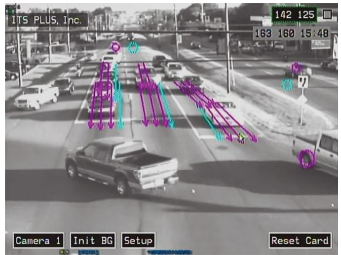
ITS Plus Dual Detection Algorithms: Circle Zones are optimized for counting and advanced detection to 1,000 feet, while Line Zones perform stop bar detection.
