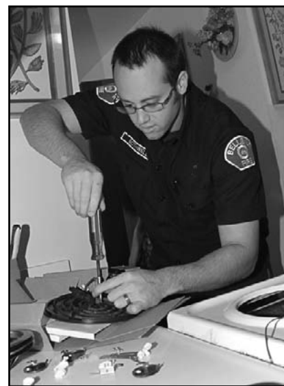
Firefighter Brandon Bothwell installs a Safe-T-Element on an electric range.
