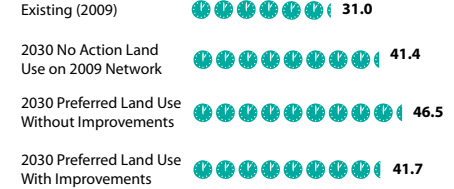
17 Total Entering Volume (TEV) in PM peak hour and average delay (seconds/vehicle)
