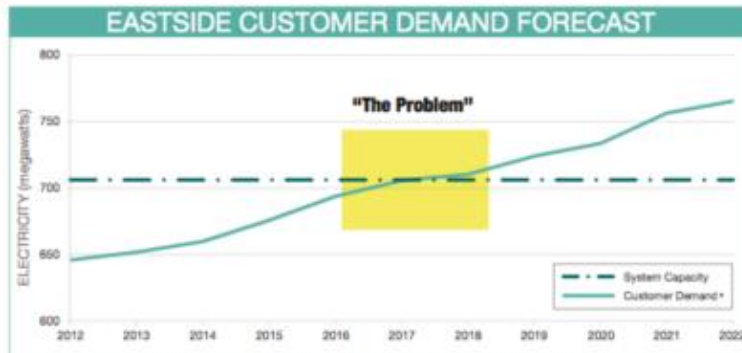
*Customer Demand assumes 100% of conservation goals are met. This chart shows customer demand with 100% conservation goals met compared to our current electric transmission system's capacity. By 2017-2018, demand will exceed our ability to provide dependable power.
