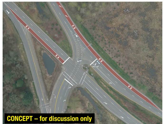
Figure 66 Running Way Improvement Project L10 and Spot Improvement Project Q11: A shoulder transit-only bypass lane would eliminate signal and queuing delay for northwest-bound on this segment of Lake Hills Connector, and a queue jump lane would assist southeast-bound buses. Both projects would require new lanes to be constructed if implemented as shown, but all existing general purpose travel lanes would be maintained.
