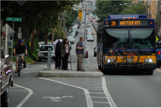
Figure 31 Transit island with in-lane bus stop.
