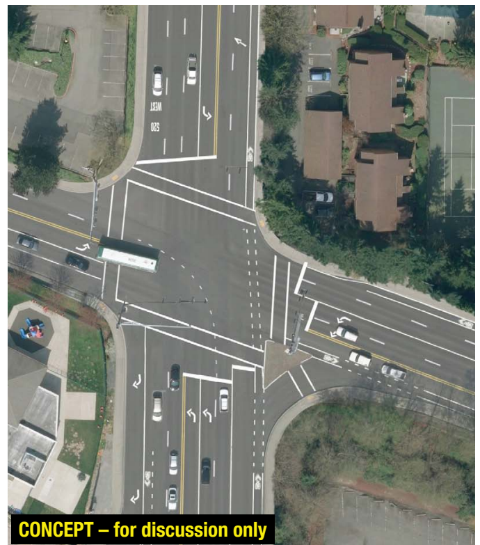
Figure 70 Spot Improvement Project Q4: Queue jump lane on 108th Ave NE for northbound buses at Northup Way. Also pictured are Running Way Improvement Projects L15 and L17 along Northup Way and 108th Ave NE, respectively. Aerial images depict roadway striping before and after lane reconfiguration. This concept repurposes existing travel lanes.
