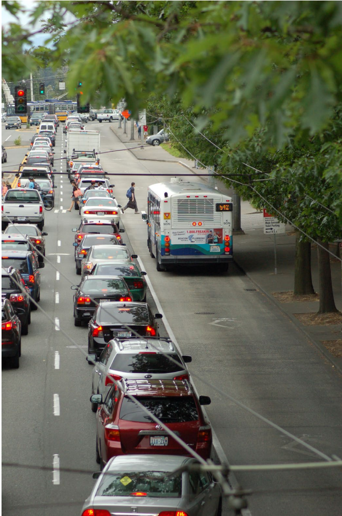
Figure 35 Bus in an HOV lane.
