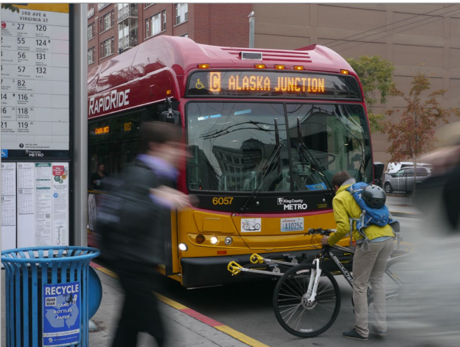
Figure 28 Unlike bull pull-outs, in-lane stops do not incur delay by requiring buses to re-enter the traffic stream.
