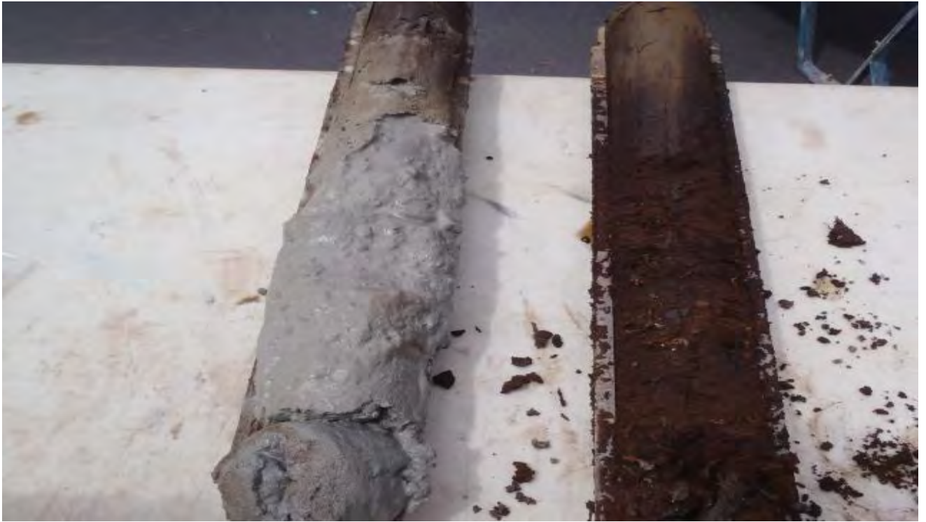
Soil sample collected with split spoon sampler from GEIMW-4- peat is visible on the right
