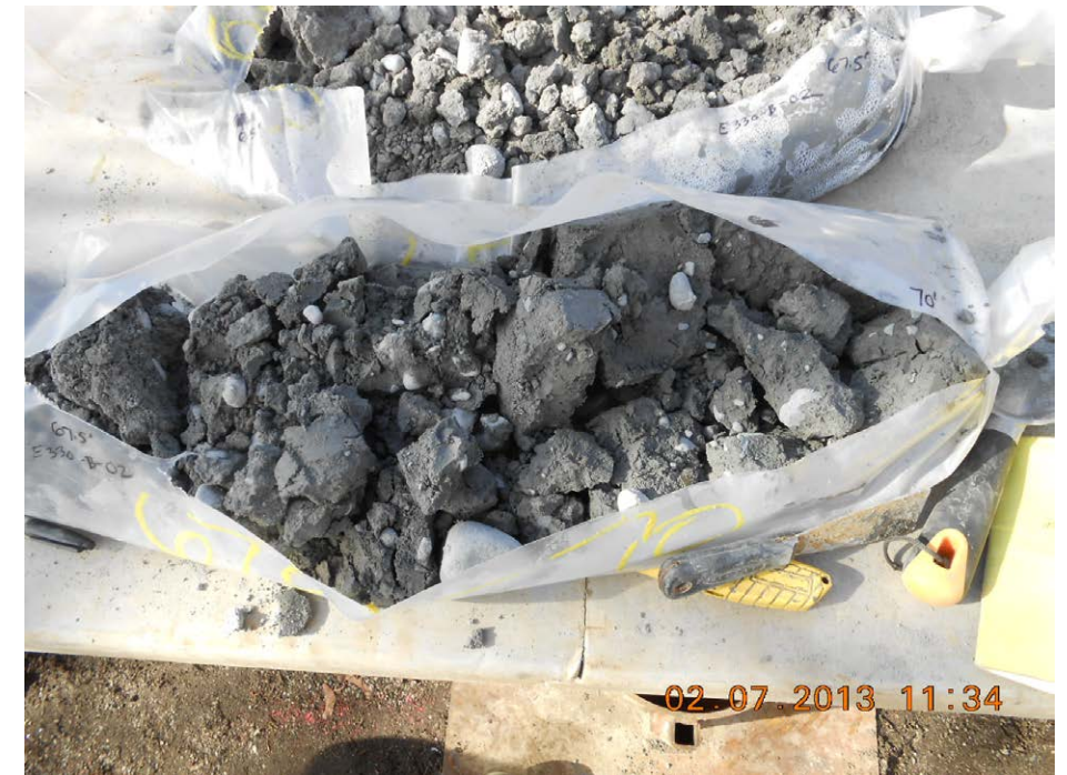
E330-B-002 67.5-70FT (END OF BOREHOLE)
