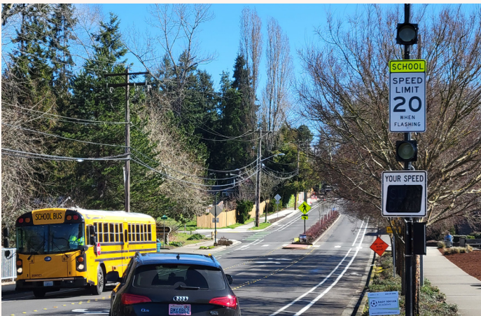
Figure 4: A new combination school zone flashing beacon and radar sign which began operation in 2023.
