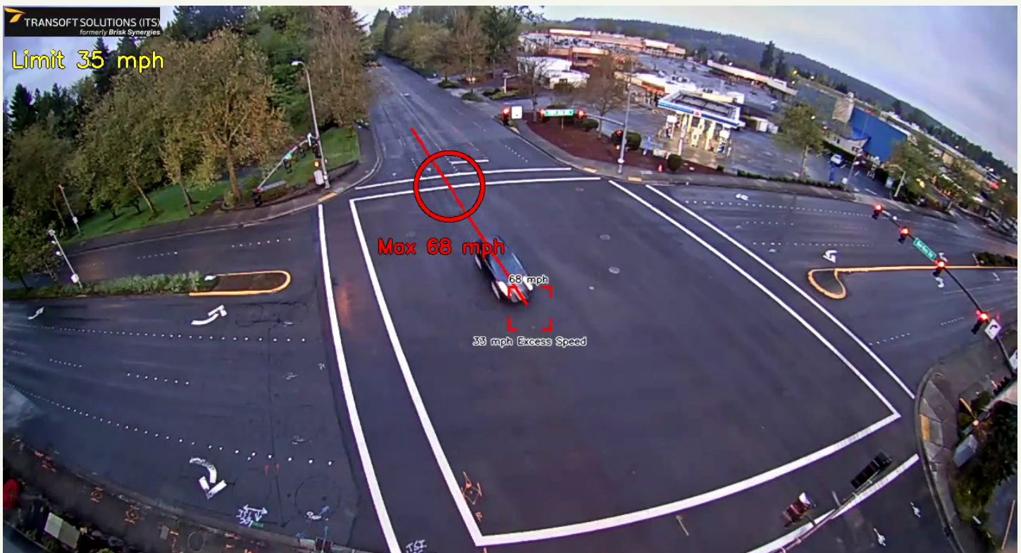
Figure 40: A road user detected through video analytics was running a red light and exceeding the posted speed limit by 33 mph through the intersection of Bel-Red Road and 148th Avenue NE. Bellevue's partnership with Transoft Solutions and Together for Safer Roads detected 8 million motorists during the one week study. Of these motorists, 870,000 (or 10.8 percent) were traveling over the posted speed limit, and half of those who were speeding drove at or in excess of 11 mph above the posted speed limit (see Speeding Analysis Report ). State regulations do not allow the use of traffic cameras to enforce speeding except in school speed zones.
