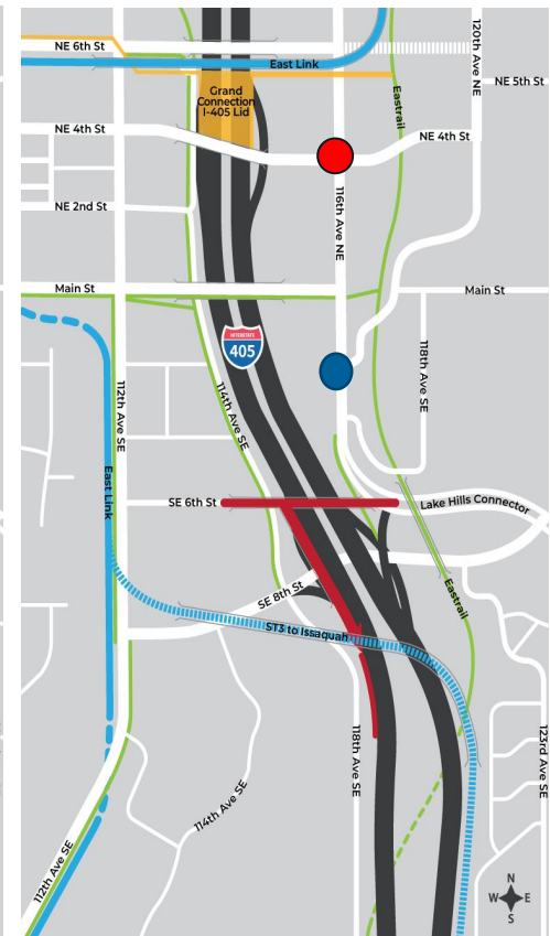
Southeast Sixth Street extension and southbound on-ramp
