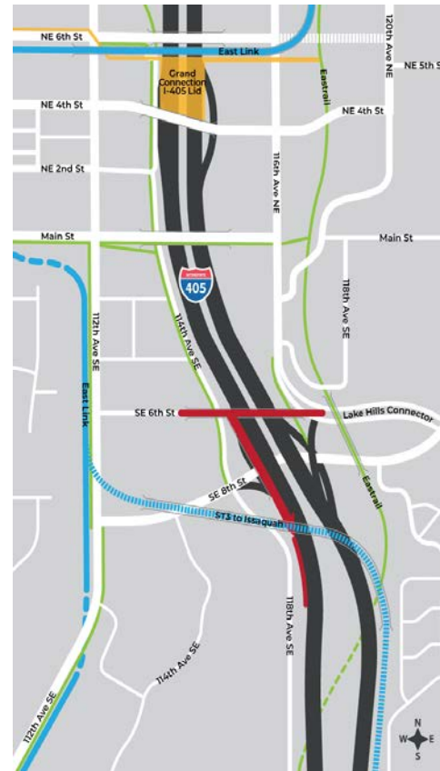
SE Sixth Street extension with southbound on-ramp
