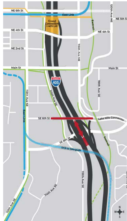
SE Sixth Street extension with direct express toll land access to/from south
