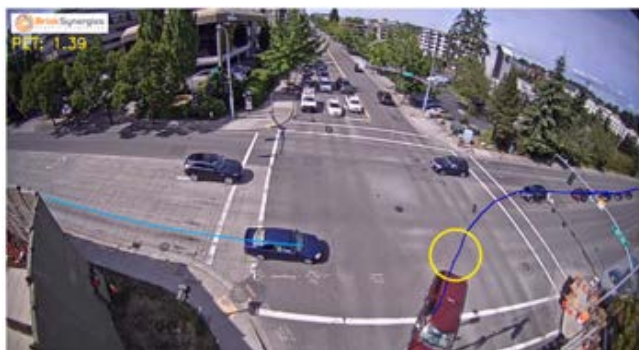
Figure 4.4 – Westbound left turning and eastbound through driver conflict at 112th Ave & Main St
