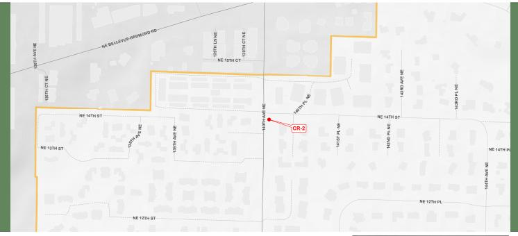
**Description:** This project would install a new PSE-owned and maintained LED street light on the Southeast corner of 140th Ave NE and NE 14th St over the existing crosswalk. On-going electricity costs would be paid for by the city.
