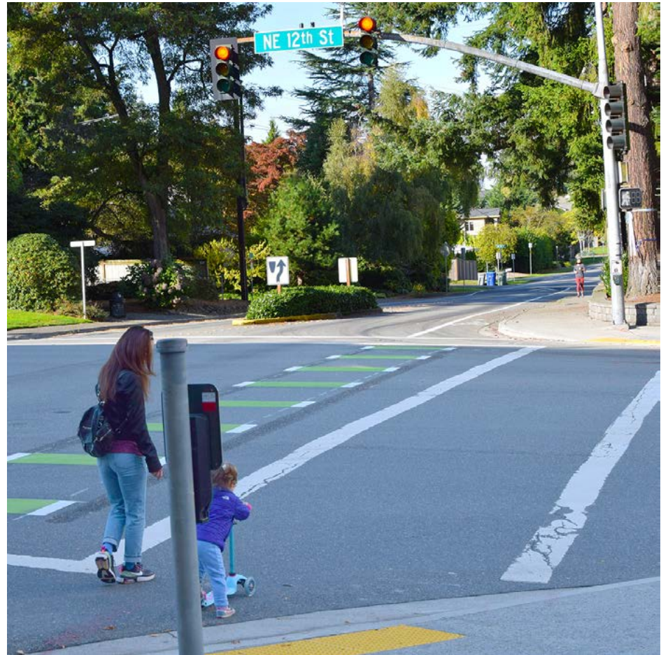
Pedestrians get a “head start” at a traffic signal modified with a leading pedestrian interval.
