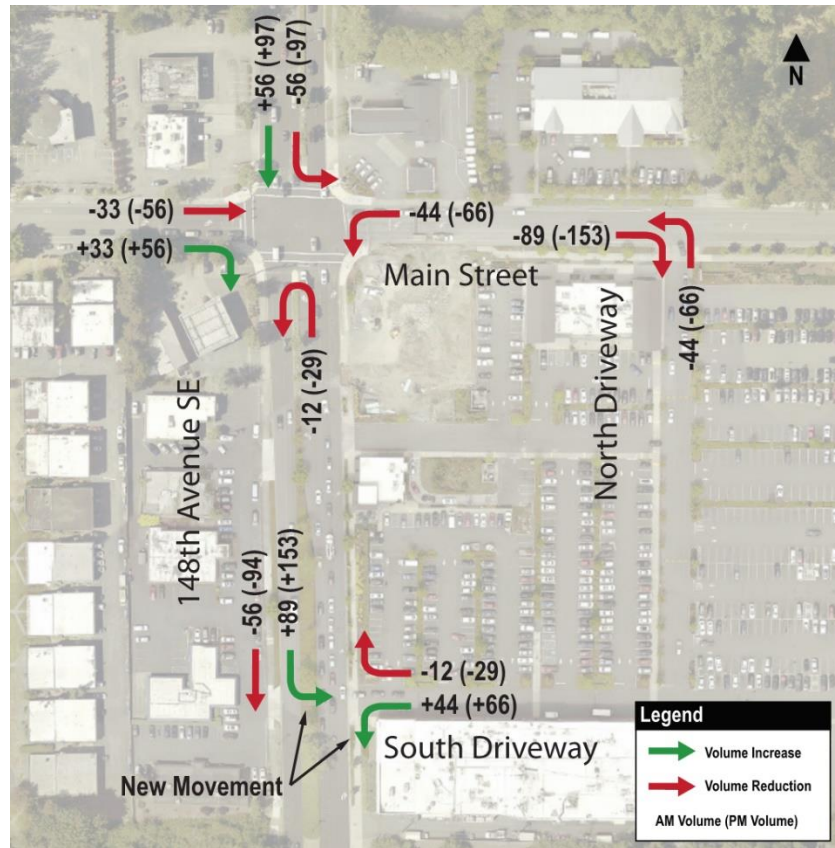
Figure 12. 2035 Traffic Diversion with Signalized South Driveway
