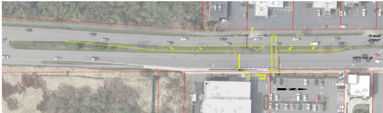
Figure 10. Limited access signal with southbound left turn lane and merge lane
