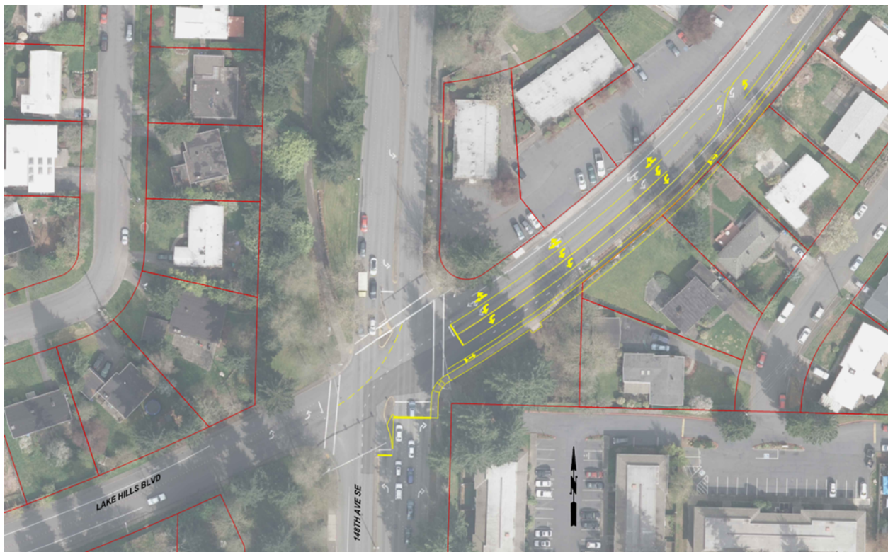
Figure 8. Recommended Alternative – Additional Westbound Left Turn Lane with Lead/Lag Operation for Westbound and Eastbound Left Turn
