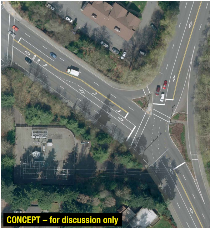
Figure 59 Running Way Improvement Projects L2, L3 and L4: Median HOV lanes on Bellevue Way SE and 112th Ave SE would improve the movement of transit vehicles through this congested Y-intersection southbound to South Bellevue Park-and-Ride. This would be achieved by constructing one lane on Bellevue Way SE and constructing a new median lane on 112th Ave SE. Aerial images depict roadway striping before and after lane reconfiguration. This concept maintains all existing general purpose travel lanes.
