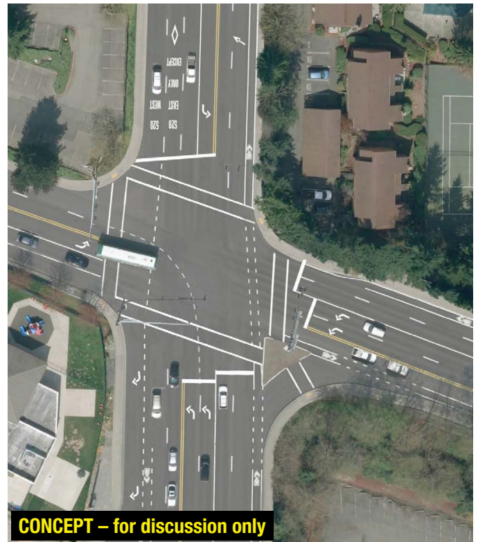
Figure 66 Running Way Improvement Project L17: Construction of a southbound HOV lane on 108th Ave NE between South Kirkland Park-and-Ride and SR-520. Aerial images depict roadway striping before and after lane reconfiguration. This concept adds one lane to the north approach relative to the WSDOT intersection reconfiguration currently being implemented. A northbound queue jump lane was also previously being considered at this intersection (see Project Q4 on page A155), but it is no longer being considered because it cannot be accommodated by WSDOT's plans.
