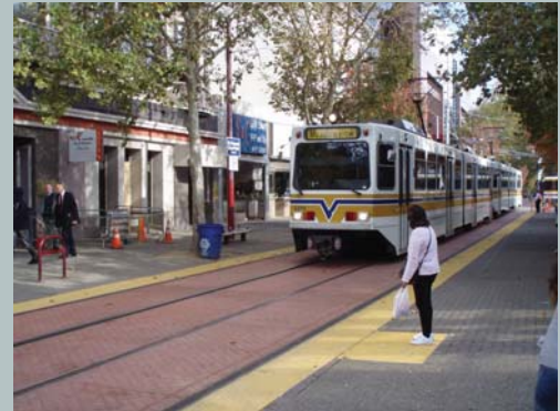
Tactile warnings and distinctive paving patterns and colors indicate to pedestrians that the zone is shared with a transit line, as shown here in Sacramento, CA. (Source: Flickr Paul Kimo)
