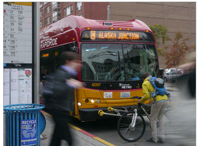
Figure 109 Unlike bus pullt-outs, in-lane stops do not incur delay by requiring buses to re-enter the traffic stream.
