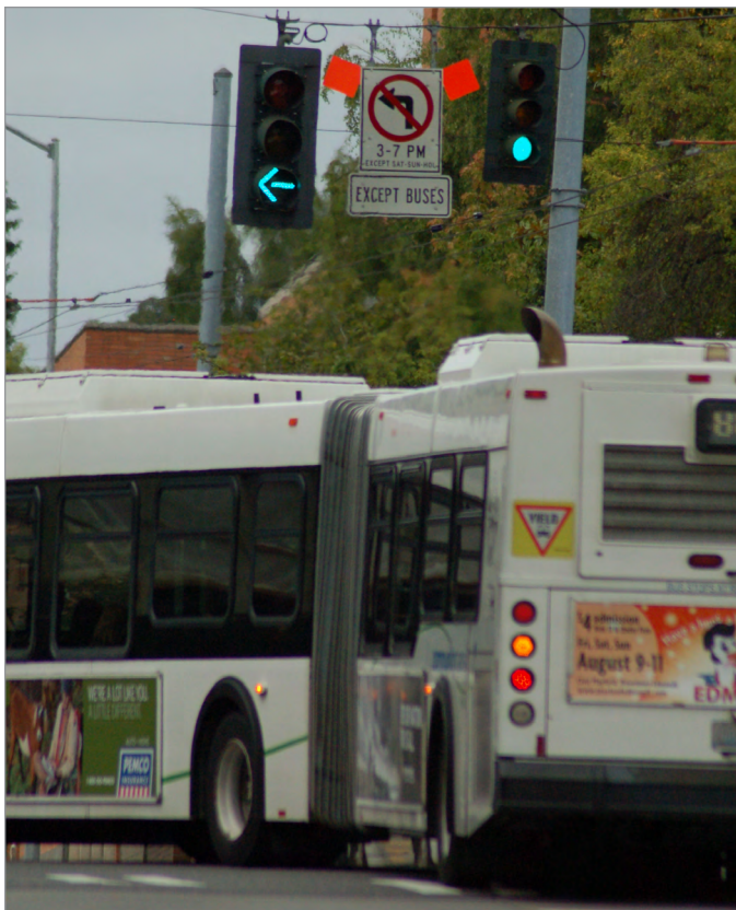
Figure 107 A bus turns during a protected phase.
