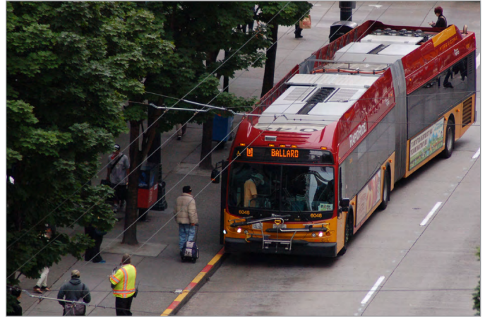
Figure 108 RapidRide bus at an in-lane bus stop.
