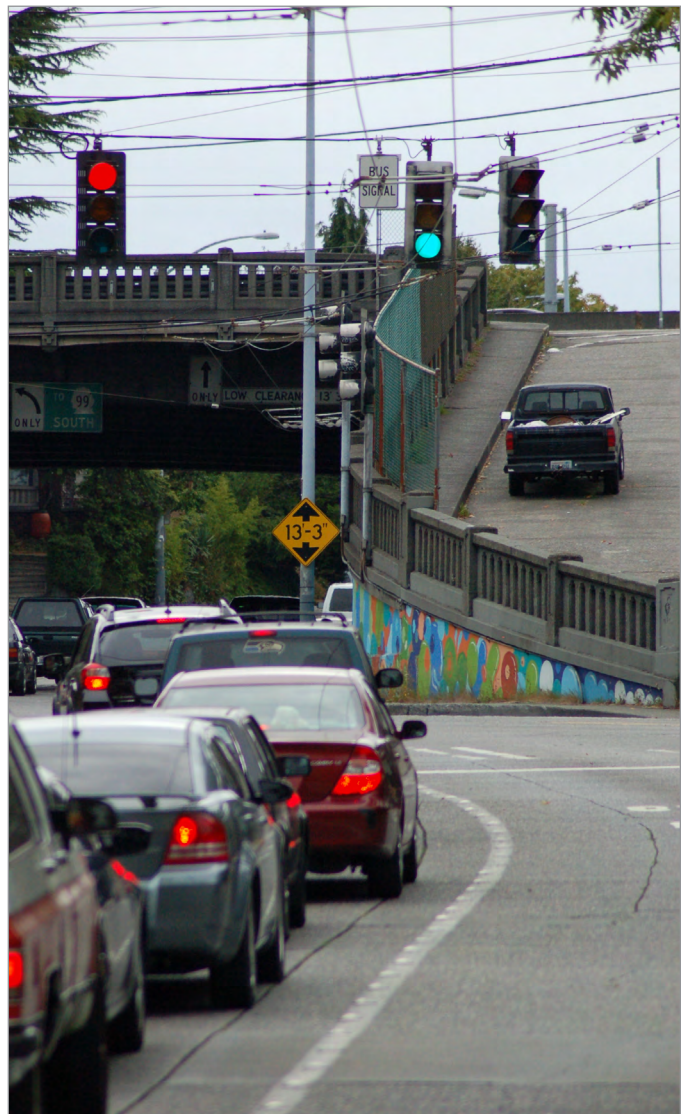
Figure 105 The bus-only queue jump lane (right signal) receives a green signal before general purpose traffic (left signal).
