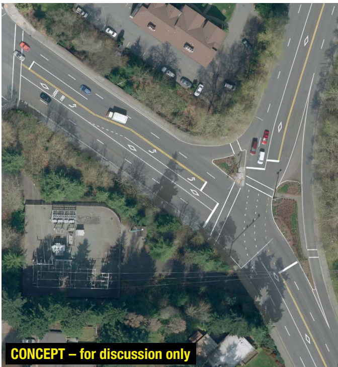
Figure 141 Running Way Improvement Projects L2, L3 and L4: Median HOV lanes on Bellevue Way SE and 112th Ave SE would improve the movement of transit vehicles through this congested Y-intersection southbound to South Bellevue Park-and-Ride. This would be achieved by constructing one lane on Bellevue Way SE and constructing a new median lane on 112th Ave SE. Aerial images depict roadway striping before and after lane reconfiguration. This concept maintains all existing general purpose travel lanes.
