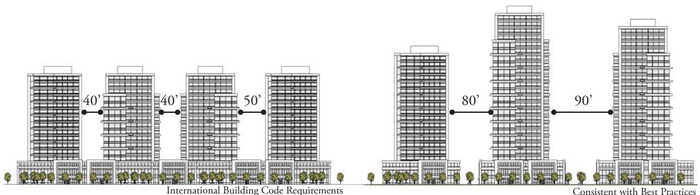
Figure 2.1 - Tower Separation Elevation
